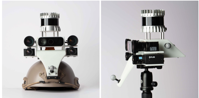
Fig. 1. We present a comprehensive set of data sequences which is recorded by a rich sensor setup placed on a versatile 3D-printed holder. It is centered around an event-based stereo camera, and further contains a regular stereo camera, an RGB-D sensor in the center, a LiDAR mounted on the top, and an IMU at the rear. The holder can be mounted on various platforms, such as a helmet as shown on the left (front view), or on a tripod as shown on the right (side view).
